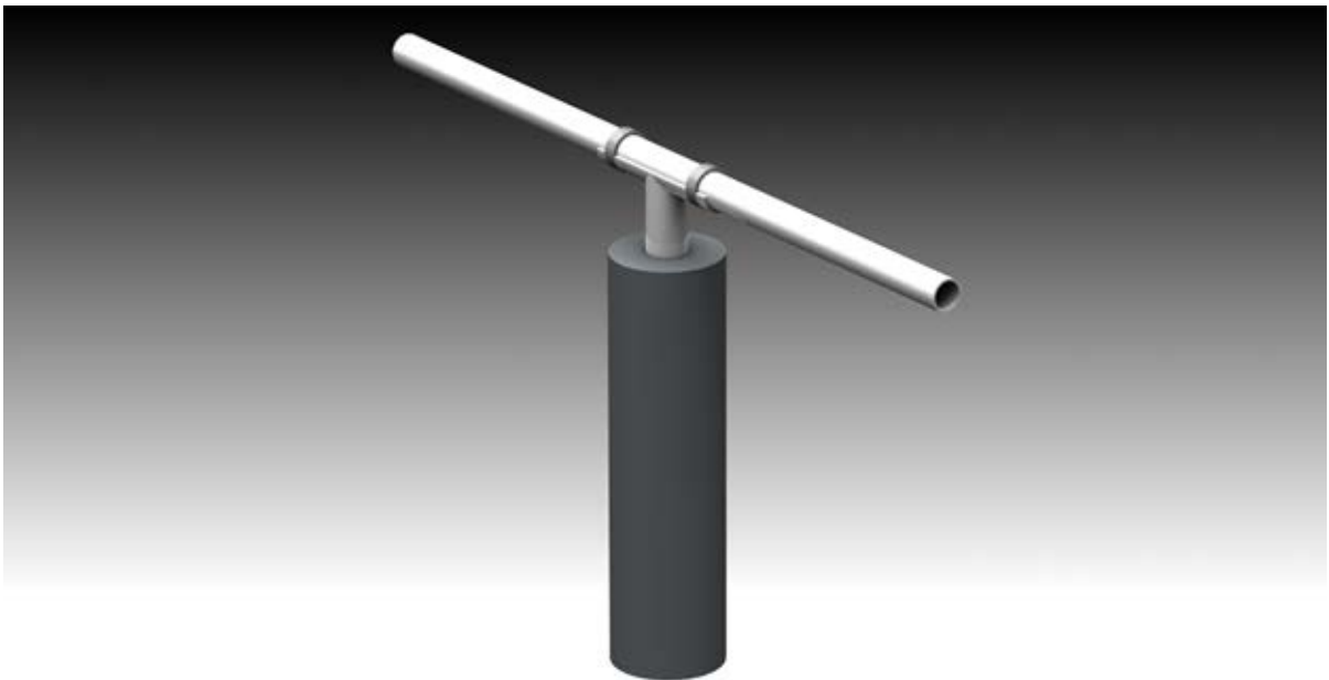
Figure 16: Uphill Pipe Supports
